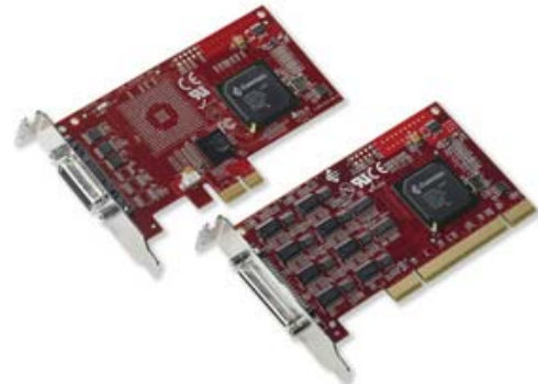
RocketPort EXPRESS cards (left) are available for PCI Express slots, while INFINITY cards (right) can be used for PCI-X or PCI connections. (Download the Hi-Res image.)
